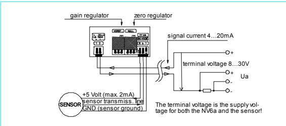
Attention! Sensor GND and NV6a GND (both at same potential) must be isolated from current loop! In a multiaxial arrangement (e.g. SW3), all sensor grounds must be isolated from each other. When ordering, look for "Sensor internally insulated, compatible with NV6a"!
